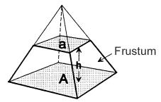
$V_F = \frac{h}{3}(A + a + \sqrt{Aa})$  where h is the perpendicular height, A and a are areas as shown
